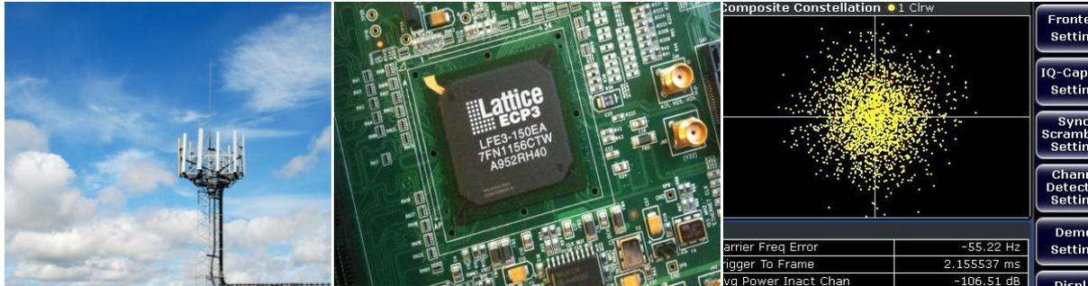
Next generation networks have increasingly adopted Remote Radio Head (RRH) technology to provide a flexible and scalable network architecture that is easy upgraded. These RRH designs include advanced signal processing technologies such as Crest Factor Reduction and Digital Pre-Distortion that optimise overall transmission efficiency and reduce net unit BOM cost.
